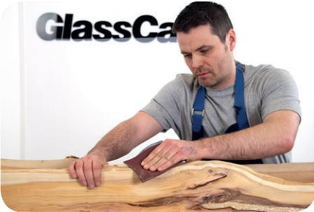
Then use some 80 grit abrasive paper to rub back any loose material left on the de-barked edge to ensure the edge is left as smooth as possible ready for the next stage.
