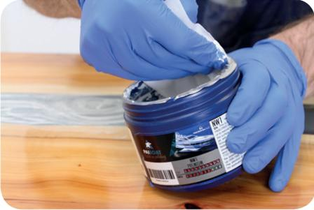
When polishing GlassCast® 50 it is extremely important that all sanding and flattening with the sander and abrasive papers has been done properly. If you find that when you start polishing the resin you can see swirls or scratches emerging in the surface of the resin, this indicates that the sanding and flattening has not been done correctly and the sanding process will need to be repeated.
