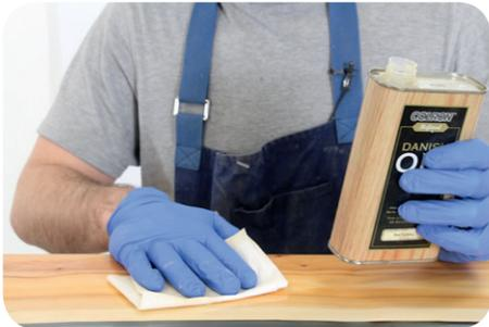
Your choice of wood finish is a matter of personal taste as different products will provide different levels of protection and varying finished appearances. It is also important to seal and finish the wood before we do the final polish of the GlassCast® river. By sealing the wood first it helps avoid the wood being marked by the polishing process; we used a clear Danish Oil.
